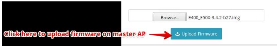
Figure 124 Upload firmware on Master AP
