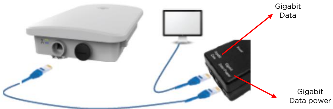
Figure 2 Installation of cnPilot to PoE adapter
