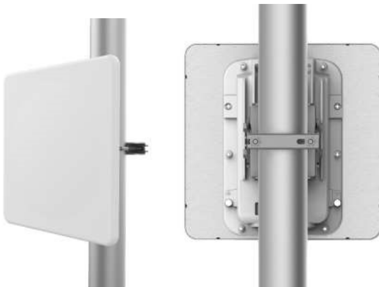
Figure 3 PTP 550 Integrated ODU (front and rear views)
