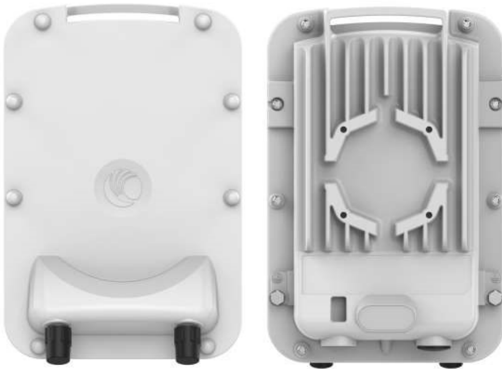
Figure 4 PTP 550 Connectorized ODU (front and rear views)
