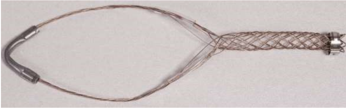
Figure 13 Cable hoisting grip
