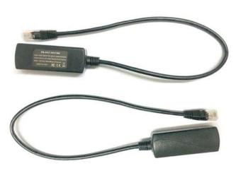
This device lets you use any 48V PoE source (including Passive PoE, Telecom PoE, 802.3af and 802.3at) to power RouterBOARD, UBNT, MTK, devices. Simply plug any 48V PoE powered ethernet cable into one port, and any 8-30V capable RouterBOARD, UBNT, MTK device into the other. This device is capable to provide high power output - up to 15W.
