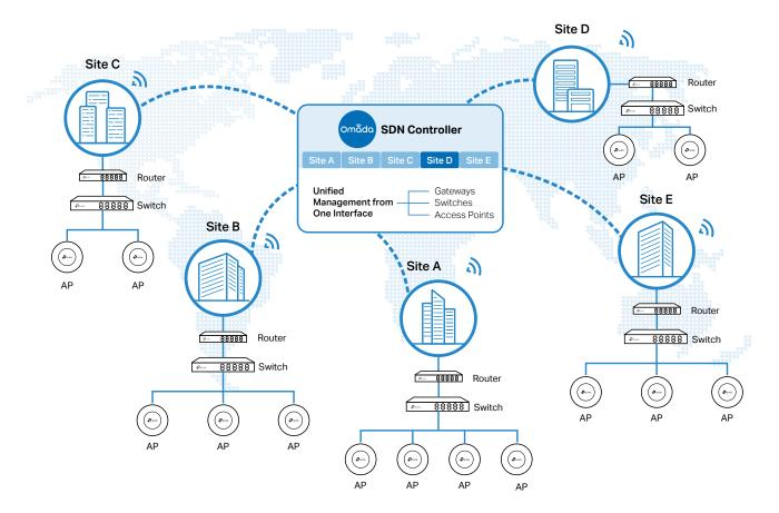
The interconnected elements that work together to deliver a unified enterprise network include: SDN Controller, gateways, switches, access points, and client devices. Beginning with a base of client devices, each element adds functionality and complexity as the network is developing, interconnecting with the elements above and below it to create a comprehensive, secure wired and wireless solution.
