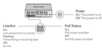
Note: For MS108GP, the Power LED is on the top right of port 8.
